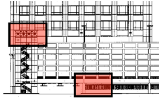
Decorative and functional railings at a parking structure. One acts as a cornice, the other secures grade-level interior space.
